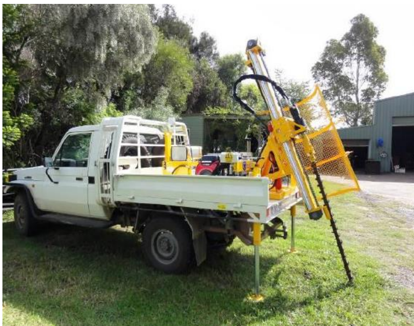
Figure 5 Standard Landcruiser tray back mounted auger
