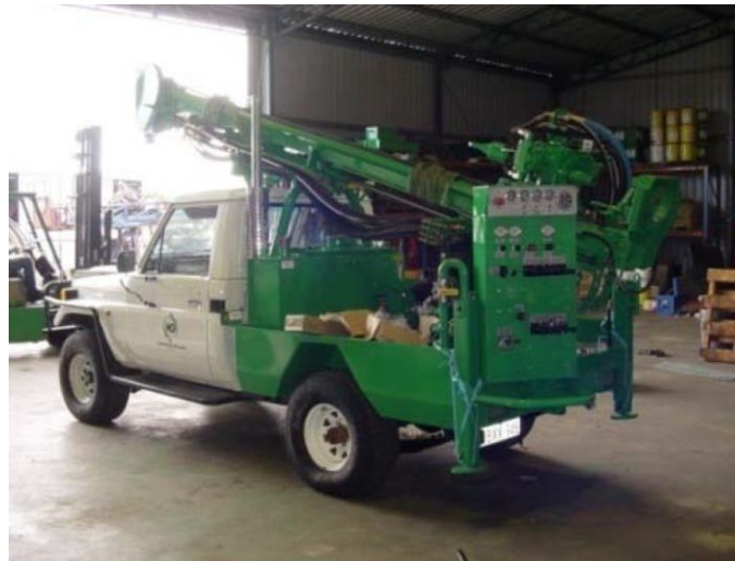
Figure 8 Landcruiser tray back mounted Mantis rig
