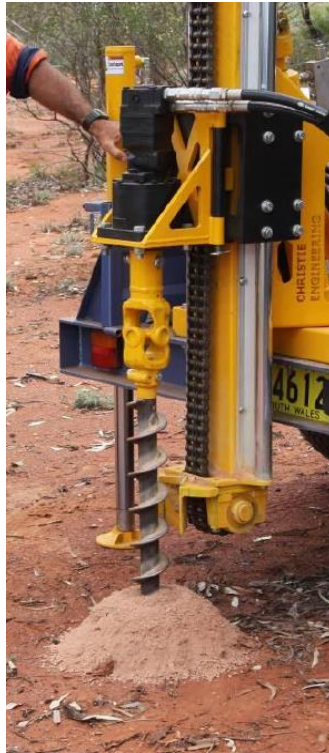
Figure 6 Traditional auger soil sampling site
