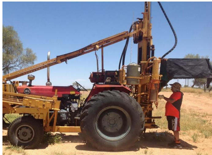
Figure 7 Tractor mounted vacuum sampling
